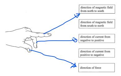
2. The diagram below shows a wire carrying a current in a uniform magnetic field. Use Fleming's Left Hand Rule to determine the direction of the force on the wire. Draw an arrow on the diagram to show the direction of the force.
