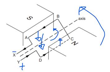
5. The diagram below shows a wire carrying a current in a uniform magnetic field. Use Fleming's Left Hand Rule to determine the direction of the force on the wire. State the direction of the force.
