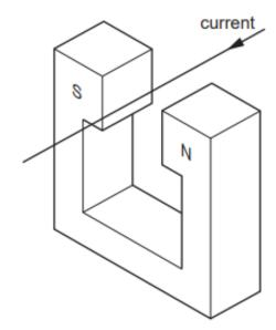
14. The diagram below shows a coil of wire carrying a current in a uniform magnetic field. By using Fleming's Left Hand Rule, draw on the direction of rotation of the coil.
