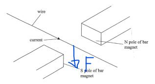
3. The diagram below shows a wire carrying a current in a uniform magnetic field. The current is going into the page. Use Fleming's Left Hand Rule to determine the direction of the force on the wire. Draw an arrow on the diagram to show the direction of the force.
